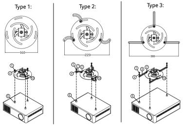
Note: It is recommended that you keep a reasonable space between the bracket and the projector to allow for proper heat distribution.
